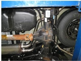
**Step 3.** Next Install the Driver and Passenger side Extension Pipe Assemblies using the supplied 2.50" clamps and fitting the hangers into the rubber insulators.
