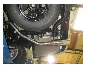
**Step 4.** Complete the installation by fastening the Driver and Passenger side Tailpipe Assemblies to the Extension Pipe Assemblies with the supplied 2.50" clamps and fit the hangers into the insulators.
