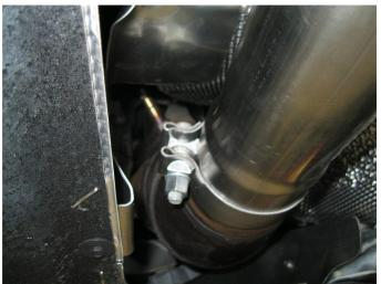
**Step 2.** Begin installation of the new system by fastening the Inlet Pipe to the outlet of the catalytic converter using the supplied 3.00" clamp.
