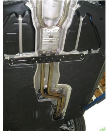
Step 1. NOTICE; to fit this exhaust system the vehicle must have a BMW M5 rear valance (P/N 51128050480) installed. To allow for extraction of the OEM system you must first remove the underside cross brace. Next loosen the clamp at the outlet of the catalytic converter. Working front to rear detach all hangers from rubber insulators and remove the system. Retain rubber insulators and clamp as they will be re-used the mount the new system.
