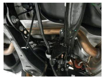
**Step 1.** It is necessary to cut the OEM exhaust to remove it from the vehicle. Locate a point above the rear swaybar with enough room to work and cut the OEM pipe.
