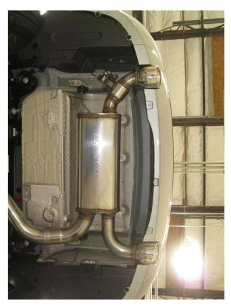
**Step 5.** Lastly, install the Extension Pipe and Muffler Assembly by fitting the hangers into the rubber insulators and fasten using the supplied 3.00" clamps. Plug the wire connector into the servo motor install factory braces.
