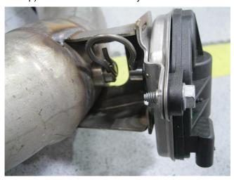
**Step 2.** Once on the OEM system is on the ground you will need to swap the servo motor from the factory control valve to the control valve on the Magnaflow Muffler Assembly. Unbolt the motor and remove the drive spring (take notice of how the drive spring is orientated as it must be re-installed the same way) and steel heat shield. Install the motor and heat shield to the valve, insert the drive spring and tighten.
