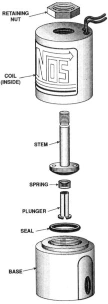
**Exploded View of a Typical Solenoid**
