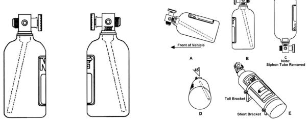
Figure 2 Nitrous Bottle Siphon Tube Orientation
