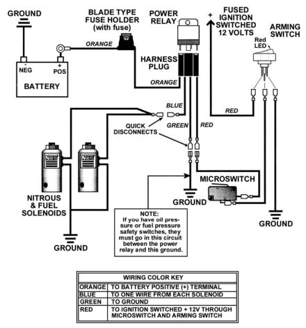
Figure 10 General Electric Wiring Diagram
