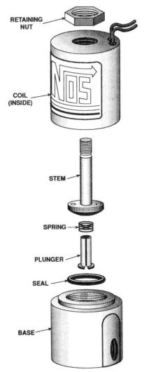
Figure 24 Exploded View of a Typical Solenoid
