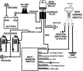
Figure 12 Electric Wiring Schematic
