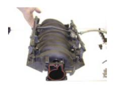
4. Now that you have removed the rail mounting bolts, lift the factory fuel rail off of the intake. Be careful as to not damage the fuel injector o-rings.
