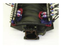
10. Before wiring up the NXL system you will need to put the fuel crossover together. First get the two Aeroquip fittings supplied in the kit, lubricate the inside of the hose ends, then slip the fittings into the hose. Be sure to butt the hose up against the coupler of the fitting. Then tighten the -AN nuts onto the NXL fuel rails and your fuel setup is complete
