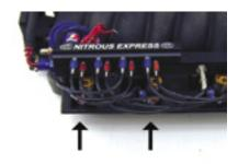
9. You may now install the nitrous and fuel lines from the rail to the nozzles. When installing start from front to back on the rail to the nozzles with the exception of the first one. If you will notice that in the third picture the front NXL nozzle on both sides of the intake, attatches to the third set of outlets. Then starting with the second one, they go from front to back, this is due to the tight radius of the hose.
