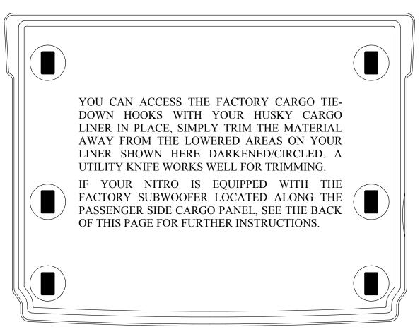
NITRO CARGO LINER SHOWN TRIMMED FOR OPTIONAL FACTORY SUBWOOFER. TO TRIM FOR THIS OPTION, SIMPLY REMOVE THE MATERIAL FROM THE RECESSED AREA MOLDED INTO THE LINER. USE THE EDGE OF THE RECESSED ARC AS YOUR TRIMMING GUIDE.
