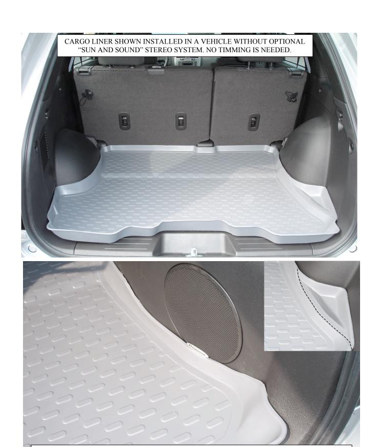
CARGO LINER SHOWN INSTALLED IN A VEHICLE WITH OPTIONAL "SUN AND SOUND" STEREO SYSTEM. YOU WILL NEED TO TRIM YOUR LINER TO ACCOMMODATE THIS FEATURE. TO TRIM, FOLLOW THE MOLDED-IN TRIM GUIDE (SEE DOTTED LINE IN INSET).
