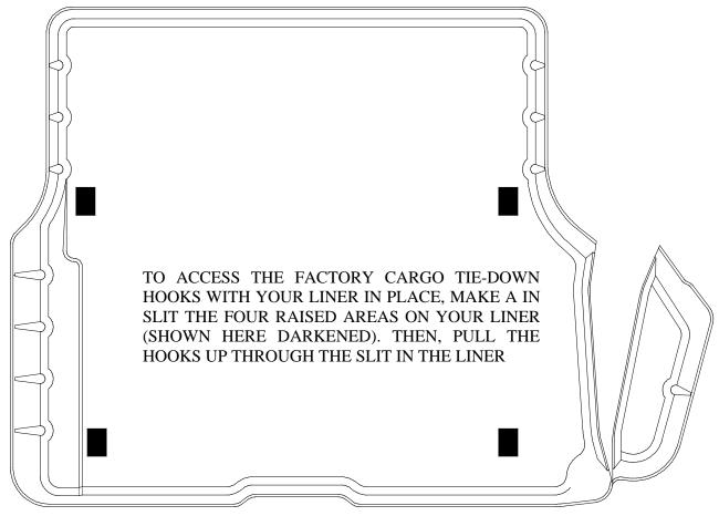
ENVOY OWNERS AND OWNERS WHOSE VEHICLE IS EQUIPPED WITH THE "ON STAR®" OPTION WILL NEED TO TRIM THEIR LINER AS SHOWN ABOVE, REMOVING THE OUTER RIGHT PORTION. TRIM ALONG THE GROOVE IN THE RAISED RIDGE AS SHOWN. A UTILITY KNIFE OR SCISSORS WORK WELL.
