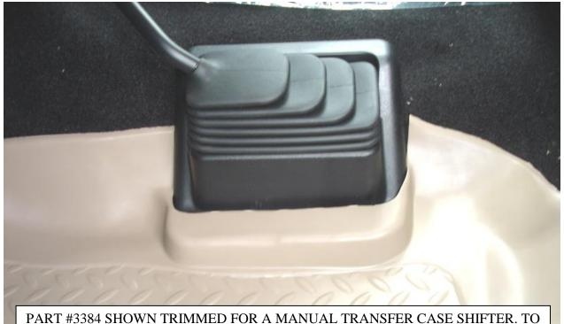
TRIM, SIMPLY REMOVE THE LOWERED SECTION ON THE LINER.
