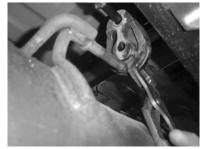
9. Remove muffler hangers from rubber isolators.
