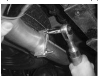
21. Align exhaust tip (D) properly and tighten clamp (G).
