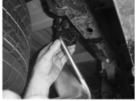
19. Insert turnout w/ tip and hanger into rubber isolator at the rear of the vehicle, near the spare tire.
