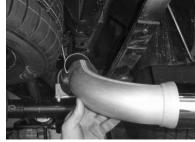
18. Install turnout w/ tip (D) at the end of tail pipe (C).
