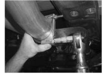
12. Install intermediate pipe (A) and secure with exhaust clamp (G).
