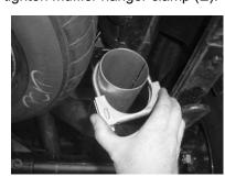
17. Install exhaust clamp (H) loosely over tail pipe (C). Do not tighten at this point.
