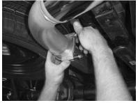
20. Position exhaust clamp (H) over slip connection on turnout w/ tip (D).
