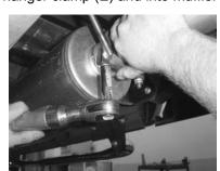
16. Align tail pipe (C) properly and tighten muffler hanger clamp (E).
