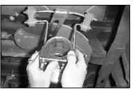
14. Slip muffler hanger (G) over end of muffler (B) and hand tighten only.
