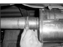
15. Install clamp (D) onto rear of muffler (#).
