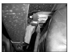
4. Using a pry bar or a pair of channel lock p remove hangers from rubber isolators at the to of the muffler.
