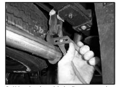
5. Using the channel lock pliers, remove the tail pipe hanger from the rubber isolator.
