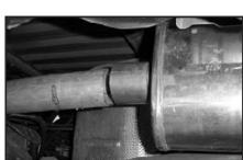
13. Insert tailpipe (C) into muffler (B).
