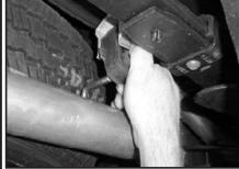
14. Install tail pipe hanger into factory rubber
