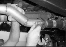
7. Using original fasteners, connect intermediat pipe (A) to the factory catalytic converter pipe.
