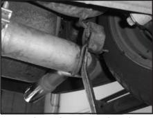
4. Using the pry bar, remove the tailpipe hangers form the rubber isolators.
