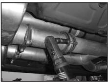
7. Align the mufflers and the tighten the fasteners that attach the intermediate pipes (A) and (B) to the catalytic converter assembly.
