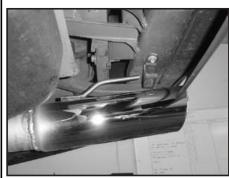
12. Install the JBA tail pipes (F) and (G) by first inserting the tip hanger in to the rear rubber isolator.
