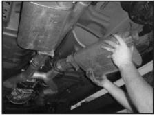
6. Install the new JBA intermediate pipes (A) and (B) and secure them to the catalytic converter assembly using the factory or supplied hardware. Now slip the JBA mufflers (C) on to the intermediate pipes (A) and (B) with the offset openings towards the middle of the car.
