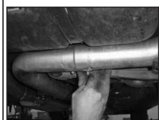
15. Position the band clamps (H) over slip connection.
