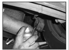
3. With the vehicle raised and properly supported, spray penetrating oil on all factory rubber isolators.
