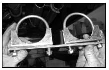
13. Assemble the new rear exhaust support bracket (G) with the supplied 3" clamps (F)
