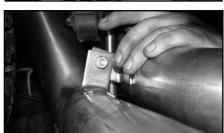
10. Insert turn out (C) and attach to turn out (D) using the supplied nut and bolt. Snug (C) and (D) together but don't fully tighten
