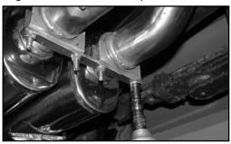
20. Finally tighten the support bracket.
