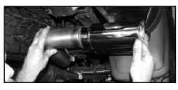
16. Align the turn outs (C) and (D) and tail pipes (E) and (B) for proper fit and clearance.
