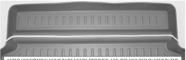
AFTER CONFIRMING YOUR PART NEEDS TRIMMED, USE THE MOLDED IN STEP IN THE PART AS YOUR GUIDE AND REMOVE THE FRONT PORTION OF THE LINER AS SHOWN. A UTILITY KNIFE OR HEAVY SHEARS WORK WELL FOR TRIMMING.
