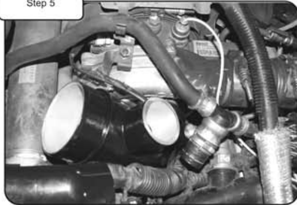
Install aFe turbo inlet tube. Ensure flange clamp fit correctly on turbo inlet tube and turbo. Do not tighten clamp.
