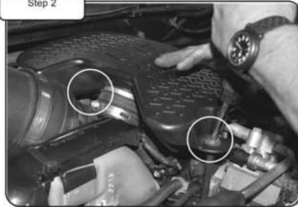
Remove resonator plenum: remove mounting screw with T30 Torx driver. Loosen clamp with flathead screw driver or 1/4" socket driver.
