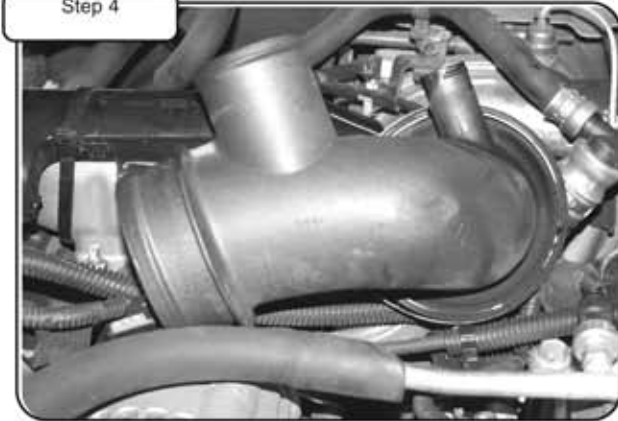
Loosen turbo inlet tube flange clamp with 5/16" socket driver. Remove stock turbo inlet tube from truck.
