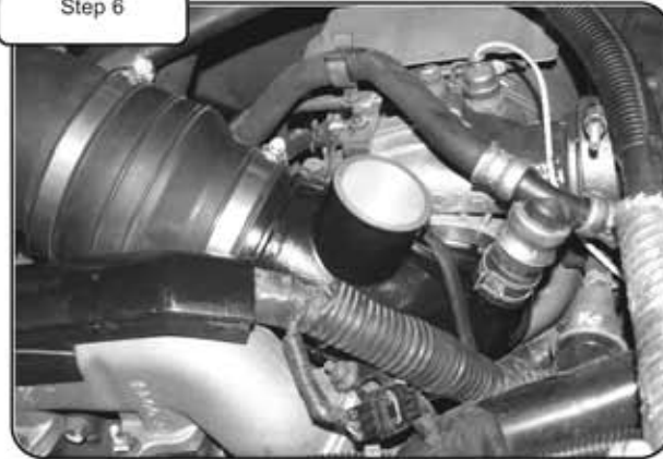
Re-attach CCV hose coupler and place clamp at original installed position with pliers. Re-attach air intake coupler clamp at aFe turbo inlet tube with flathead screw driver or 5/16" socket driver. Tighten flange clamp from Step 5.
