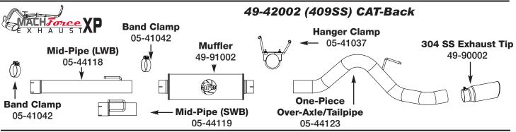
**Step 1:** (Read Instructions prior to installation) Loosen band clamp from the cat rearward. Remove your stock exhaust from the rear of your truck working your way forward. It may be necessary to cut the pipes if the slip joints are stuck. Take caution not to damage the factory isolation mounts as they will be reused.
