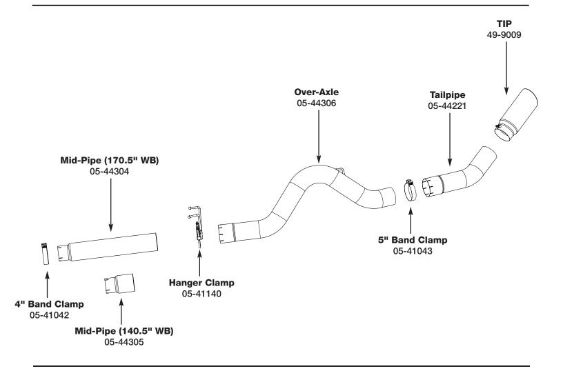
**Step 1:** (Read Instructions prior to installation) Remove your stock exhaust from the rear of your truck working your way forward. It may be necessary to cut the pipes if the slip joints are stuck. Take caution not to damage the factory isolation mounts as they will be reused. It is recommended to not fully tighten the clamps until the entire system has been installed.
