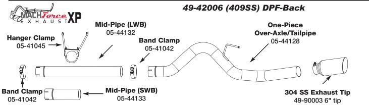
**Step 1:** (Read Instructions prior to installation) Loosen band clamp at rear of particulate filter before muffler. Remove your stock exhaust from the rear of your truck working your way forward. Take caution not to damage the factory isolation mounts as they will be reused. It is recommended to not fully tighten the clamps until the entire system has been installed.
