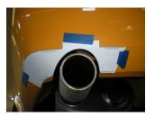
4) Because there is no cutout in the rear valance for the left side tailpipe, it will be necessary to make a new cutout. Follow the instructions on the attached template to properly align and make the cutout.
