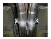
6) Place a 2¼" clamp onto the slip-fit of over-axle pipe **#16679S** and slide onto the back of the right Scavenger outlet and support with a stand. Repeat this step with the left over-axle pipe **#16680S**.
