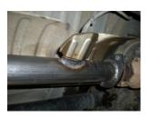
4) Connect the flange on inlet pipe **#16709S** to the flange behind the catalytic converter. Be sure to replace the gasket between the two flanges. Use the included 3/8" bolts, nuts and washers to secure the two flanges together. Use the included 5/16" x  $\frac{3}{4}$ " bolts and lock washers to re-install the O2 sensor to the inlet pipe.
