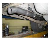
4) Place both tailpipes **#16793S** and **#16794S** up over the rear axle and connect the hangers on the tail pipes to the rubber mounts installed in Steps 2 & 3 above.
