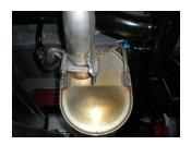
2) To make the removal of the stock system easier, using a hacksaw or sawsall cut the stock tailpipe off where it exits the muffler. Remove the hanger at the rear of the tailpipe from the rubber mount on the vehicle and set the tailpipe aside. This step is not mandatory, but makes removal easier. There are retainer clips on the ends of each of the hangers that will need to removed with pliers to allow disassembly.
