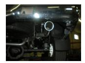
11) Slide either the side exit pipe #16317\$ or the rear exit pipe #16397\$ on the ends of both over-axle pipes. Place a 2 1/2" clamp onto these slip-fit connections. Tighten enough to hold, but still allow for adjustment. Place the two stainless tips #\$T396 onto the exit pipes and tighten the clamps enough to hold, but still allow for adjustment. Rotate the exit pipe and tip to the desired distance from the fender or bumper and so angle cut on tips are in the desired location.
