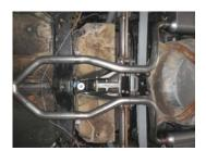
2) Place a provided clamp onto both outlets of X-pipe assembly **86171S**. Place the expanded end of mid pipe **86231S** onto the right outlet of the X-pipe assembly. Rotate the pipe up into position and support the rear of the pipe with a stand. Tighten the clamp enough to hold, but still allow for adjustment. Repeat this step on the left side of the vehicle with pipe **86232S**.
