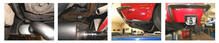
4) Place one of the supplied **HA602** rubber mounts onto the wire hanger of left muffler assembly **842456-352.** Place a provided clamp onto the muffler inlet, then place the assembly onto the back of the mid pipe and slide the two fully together. Support the muffler with a stand. Using a supplied 3/8" bolt, nut, washer and lock washer, bolt the **HA602** hanger to the hole in the frame above the muffler outlet.
