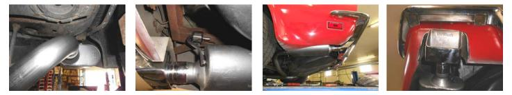
5) Adjust the position of the pipes and mufflers to provide a satisfactory fit. A minimum of 3/4" clearance around all parts of the system must be maintained; while also keeping suspension travel and vibration in mind. Tighten all clamped connections down securely.
