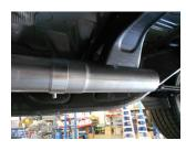
2) If installing the system on a Crew Cab truck with a 6.5' bed, place extension pipe **#TB700S** onto the back of the **#26401S** inlet pipe, place a provided clamp onto the slip-fit and tighten enough to hold in position. This extension pipe will not be used on Double Cab or Crew Cab-5.5' bed models.
