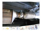
1) Place inlet pipe assembly **#26401S** into position onto the ball connection behind the catalytic converter. Reinstall the clamp onto the ball connection and tighten enough to hold, but still allow for a small amount of adjustment. Connect the hanger on the pipe to the rubber mount on the vehicle.
