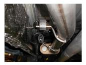
5) For Crew Cab - 6'-4" bed models place a provided 3 ½" clamp onto the expanded end of extension pipe **36062S**, place onto the back of the inlet pipe and connect the hanger on the pipe to the rubber mount on the vehicle. Tighten the clamp enough to hold but still allow for adjustment.
