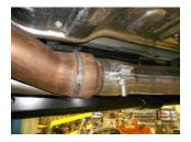
4) Place a provided 3 ½" clamp over the expanded end of inlet pipe **#36061S**, then place onto the stock front pipe just behind the catalytic converter. Be sure to line up the notch in the pipe with the tab on the front pipe. Connect the hanger on the pipe to the rubber mount on the vehicle and tighten the clamp enough to hold but still allow for adjustment.
