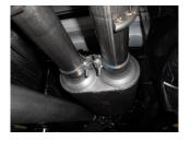
9) Install a provided 3" clamp onto the left muffler outlet. Place the front section of the left side tailpipe **#26466S** into the left side muffler outlet and connect the hanger on the pipe to the rubber mount on the vehicle. Tighten the clamp enough to hold, but still allow for adjustment. Place a second 3" onto the back of this pipe in preparation for the next step.
