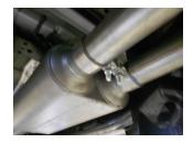
8) Install a provided 3" clamp onto the right muffler outlet. Place the right side tailpipe **#26465S** into position over the axle and slip into the right side muffler outlet, while at the same time, connecting the hangers at the front and rear of the pipe to the rubber mounts on the vehicle. Tighten the clamp enough to hold, but still allow for adjustment.
