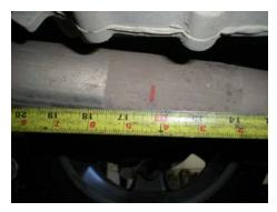
2) Begin by measuring back 16 ¼" from the edge of both factory mufflers and make a mark on the pipes (see photos above). Once you have double checked that the measurements are correct, cut both pipes through at the marks. Remove the two hangers on each tailpipe assembly from the rubber mounts on the vehicle and remove the tailpipe assemblies from the vehicle. Carefully deburr the end of the pipes with a file or die grinder.
