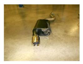
3) Place the new Flowmaster muffler units next to the factory exhaust system and swap the front and rear hanger mounts from the stock mufflers to the Flowmaster assemblies. Also, place a provided 3.00" clamp onto the inlet of each muffler assembly. Tighten the clamp just enough to hold in place.
