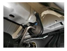
3) Using a 13mm wrench, unbolt the two hangers just behind the rear differential from the cross member. Now, with the help of an assistant, carefully lower the center stand and slide the exhaust system forward and out of the rear hanger mounts. Lower the system to the floor leaving the front hangers attached. Finally, remove the two hanger mounts at the rear of the vehicle from the rame using a 13mm wrench. As you remove them, place them with the factory muffler from the corresponding side.
