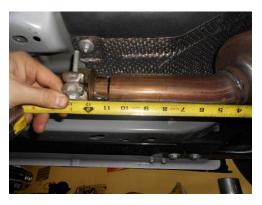
4) Begin by measuring back 11" from the bottom case weld on both catalytic converters as shown in the photos above and make a mark on both pipes. Support the exhaust system behind the area to be cut, then once you've double checked that the measurements are correct, cut both pipes at the marks. Note: Due to the closeness of the pipes to the floor of the vehicle, use caution when cutting! Carefully deburr the end of the pipes where cut with a file or die grinder.
