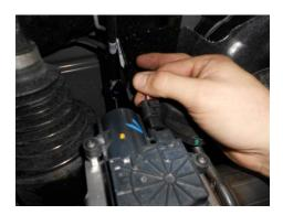
8) Reconnect the two electrical plugs removed in step 2 of the removal instructions back onto the tailpipe actuators now installed on the new Flowmaster tailpipes.
