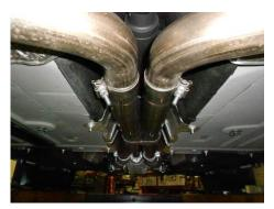
5) Begin the installation by placing a supplied 2-3/4" clamp onto each of the inlets of the Scavenger pipe #26522\$. Then place the Scavenger pipe onto the back of the stock head pipes (the offset outlet pipe should be oriented to the right side). Level and center the assembly in the drive line tunnel and support with a stand. Tighten the two clamps enough to hold, but still allow for adjustment.
