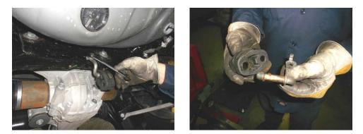
3) To install the new Flowmaster system you will need to remove the factory hanger located on the cross member just behind the rear differential. After unbolting the hanger, remove the rubber isolator from the hanger mount, the rubber isolator and the bolt/washer securing the hanger will be reused with the Flowmaster system.
