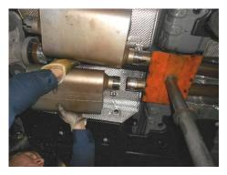
5) Place a supplied 2 ½" clamp onto the inlet of each **#842546-Z** muffler. Then fully slide the mufflers onto the back of the Scavenger pipe assembly and support with stands. Level the mufflers and tighten the clamps enough to hold, but still allow for adjustment.
