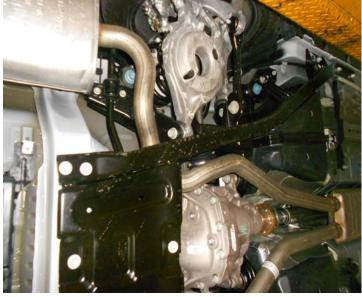
2) On convertible model vehicles, the body braces show in the photos above will need to be removed in order remove the factory system and install the Flowmaster system. Starting at the front of the right side (passenger) brace, loosen the front bolt and then work your way to the rear of the vehicle removing the next eight bolts, lower the brace from the vehicle. Repeat this step on the left side of the vehicle with the six bolts on that side.
