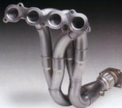
Skunk2's stainless-steel header uses a Tri-Y design with a step in the primaries; Skunk2 claims 9 hp from just this mod.
