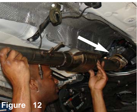
Figure 12 the primary section with the catalytic converter is aligned to the test pipe.
