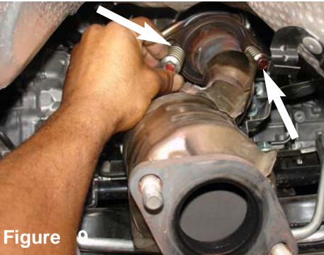
Figure 9 Tension bolts are removed from the primary catalytic converter. Once you have removed the tension bolts continue to pull the catalytic converter.
