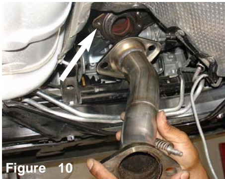
Figure 10 The new test pipe is aligned to the header exhaust as shown above.
