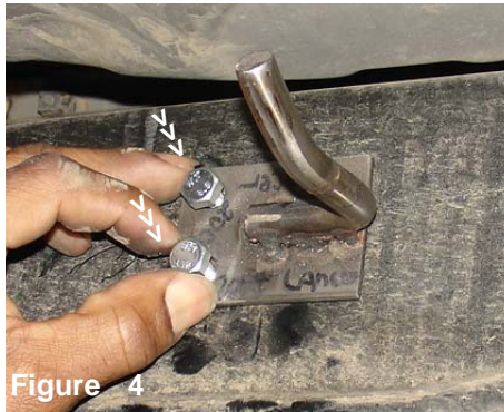
Figure 4 The two m8 bolts in this kit are used to secure the bracket in place.
