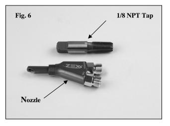
We've also enclosed a tap (Fig. 6) should you desire to mount the nozzles directly into a metal air intake tube. Just drill an 11/32 inch hole where you want to thread-in the nozzle, tap the hole and install the nozzle.
