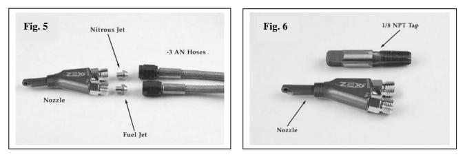
your engine. Install the nitrous nozzle so that the spray is in the direction of airflow. We've enclosed a tap (Fig. 6) should you need to mount the nozzle in a metal duct. Just drill a 11/32 inch hole where you want to mount the nozzle, tap the hole and install the nozzle. Once the nozzle is installed, place the appropriate tuning jets in the nozzle and attach the 3-foot long, -3AN hoses to the nozzle jet fittings and the nitrous management unit (Fig.5).
