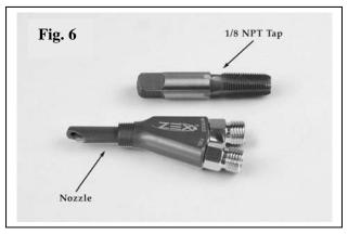
need to mount the nozzle in a metal duct. Just drill a 11/32 inch hole where you want to mount the nozzle, tap the hole and install the nozzle. Once the nozzle is installed, place the appropriate tuning jets in the nozzle and attach the 3-foot long, -3AN hoses to the nozzle jet fittings and the nitrous management unit (Fig.5).
