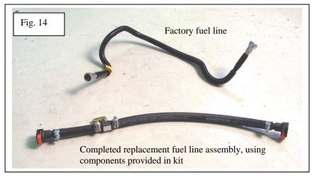
D. Attach the 4 ft. -4AN fuel line to the 90 deg. -4AN fuel fitting on the inline tee. Attach the other end of the fuel delivery hose to the nitrous management unit fuel inlet fitting.
